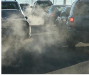
Fuel emissions contain harmful chemicals such as hydrocarbons, carbon dioxide, and nitrogen oxides.
